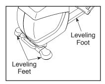
If the frame of the elliptical flexes during use, turn the leveling foot under the center of the frame until the flexing is eliminated.
