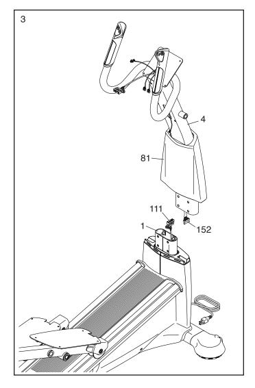
4. **Tip: Avoid pinching the wires.** Slide the Upright (4) onto the Frame (1).
