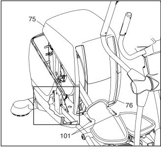
Next, tighten the M8 Nut (122) on the J-bolt (139) one half turn.
