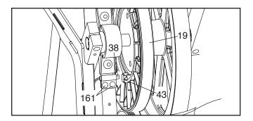
Next, rotate the Large Pulley (19) until a Magnet (43) is aligned with the Reed Switch (38). Slide the Reed Switch slightly toward or away from the Magnet. Then, retighten the M4 x 12.7mm Flange Screws (161).
