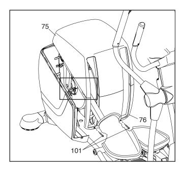
Next, see EXPLODED DRAWING A on page 29. Remove the four M4 x 16mm Screws (101) from the Pulley Cover (15), and then remove the Pulley Cover. It may be necessary to disconnect the wires (not shown) at the top of the Pulley Cover.
