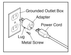
The temporary adapter should be used only until a properly grounded outlet can be installed by a qualified electrician.
