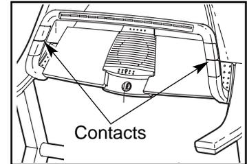
**Avoid moving your hands.** When your pulse is detected, two dashes (--) will appear in the Calories/Pulse display, and then your heart rate will be shown. **For the most accurate heart rate reading, continue to hold the contacts for about 15 seconds.**
