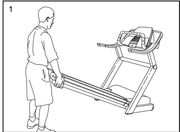
2. Hold the treadmill frame firmly with your left hand. Using your right hand, pull the latch knob to the right and hold it. Raise the treadmill until the pin on the latch knob is aligned with the hole in the left handgrip. Then, release the latch knob. **Make sure that the latch knob is fully released so the pin is fully inserted into the hole in the left handgrip.**
