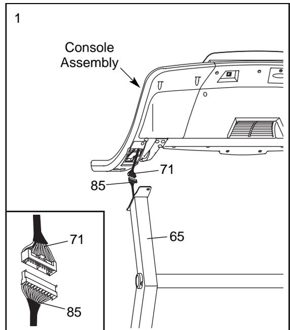
2. Insert the excess Wire Harnesses (71, 85) into the right Upright (65).
