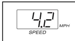
Note: The console can display speed and distance in either miles or kilometers. To find which unit of measurement is selected, hold down the Stop button while inserting the key into the console. An “E” for English miles or an “M” for metric kilometers will appear in the Speed display. Press the Speed increase button to change the unit of measurement. When the desired unit of measurement is selected, remove the key. **Note: For simplicity, all instructions in this section refer to miles.**
