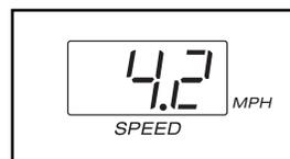
cise, change the speed of the walking belt as desired by pressing the Speed increase and decrease buttons. Each time a button is pressed, the speed setting will change by 0.1 mph; if a button is held down, the speed setting will change in increments of 0.5 mph.
