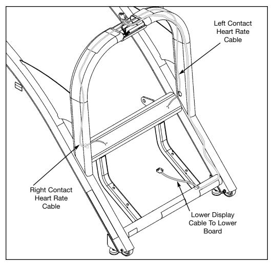
Figure 34 **NOTE:** Frame only shown for cable routing.
