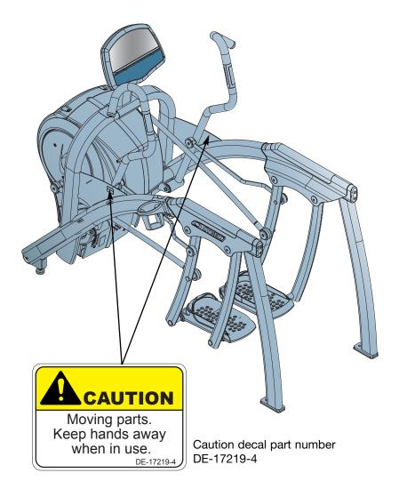
**NOTE:** This decal is located on both sides of the unit in a total of two locations.
