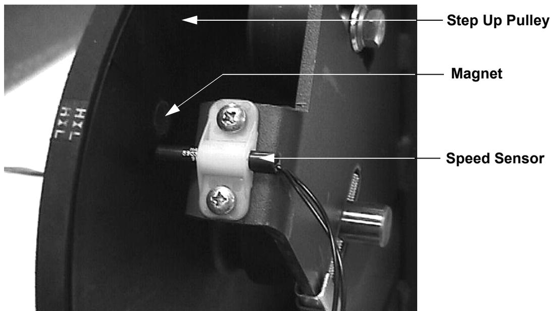
6. For serial codes F8 and SS, position the speed sensor at its mounting position and set the gap between the end of the speed sensor and the step up pulley at approximately 1/8 inch. Replace the hardware that secures the speed sensor to the drive unit. Torque the speed sensor screws to 27 in./lbs.
