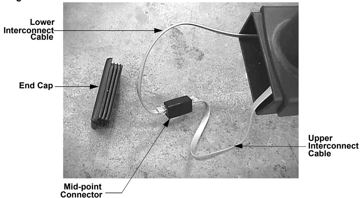
5. Disconnect both cables from the mid-point connector and replace the mid-point connector with a known good mid-point connector. If the mid-point connector does not correct the problem, replace the original mid-point connector and continue with step 5.
