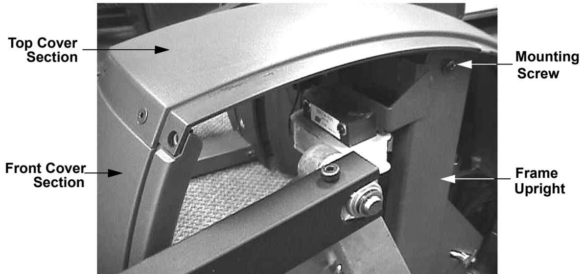
7. If all four cover sections have been removed, first replace the frame cover and front cover section, then the top cover section and then the left and right cover sections as described below.
