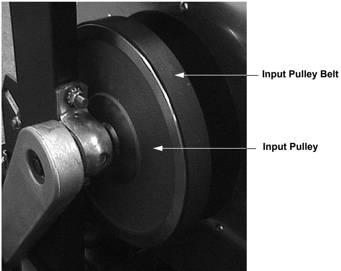
12. Slide the step up and input belts onto the input drive assembly as you set the input drive assembly in its mounting position in the drive unit.
