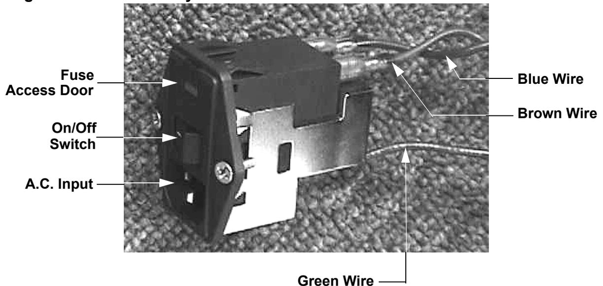
3. Remove the blue wire from terminal D, the brown wire from terminal A and the green wire from the ground terminal of the power entry module.
