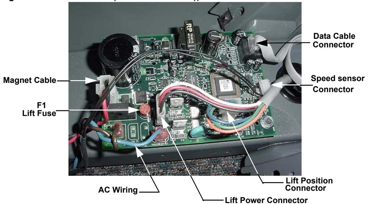
11. Remove the AC wiring, interconnect cable, speed sensor wiring and magnet cable from the lower PCA.
