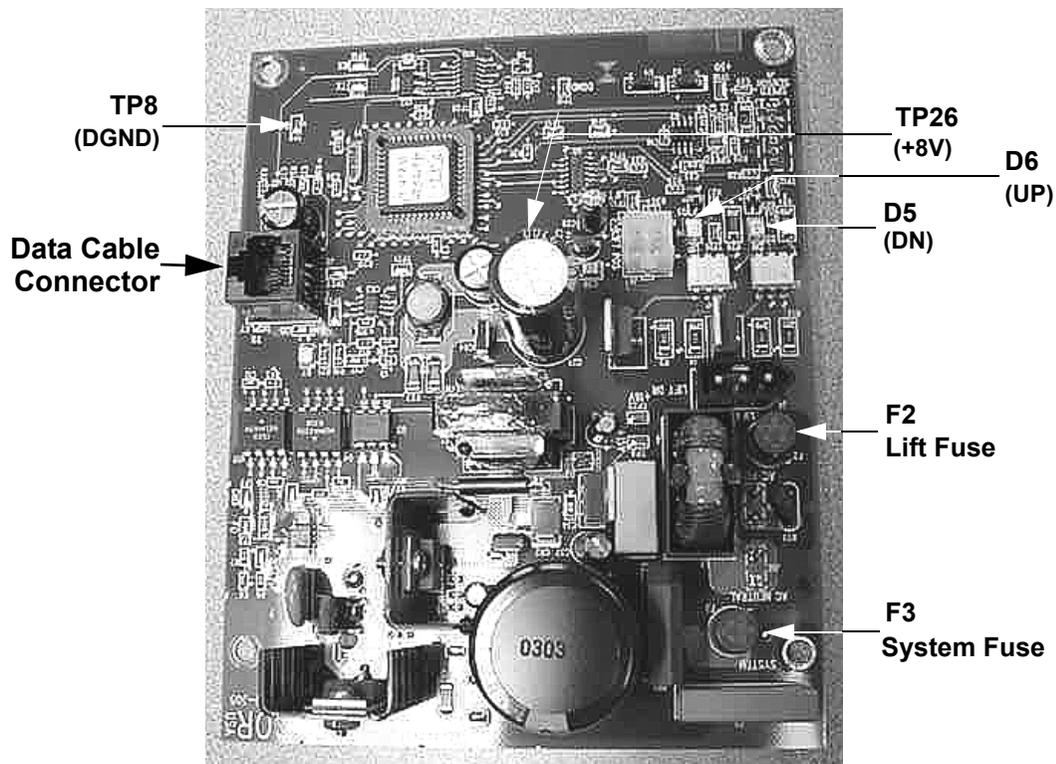
**Diagram 6.6 - Lower PCA (Serial code A998)**
