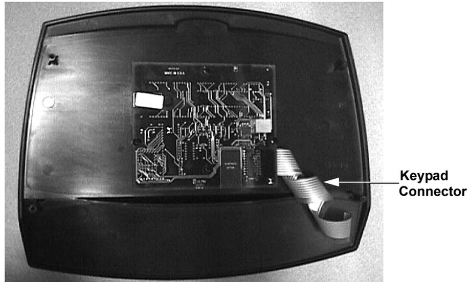
7. Position the replacement upper PCA at its mounting location on the display housing front panel (refer to Diagram 7.3). Replace and tighten the upper PCA mounting screws.
