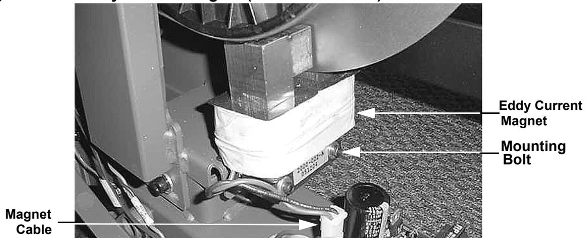
12. Set the replacement eddy current magnet in its mounting position and fasten it with the hardware removed in step 11. Torque the eddy current mounting bolts to 47 inch pounds.
