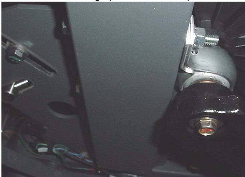
10. Thread and hand tighten the pillow block mounting nuts onto the mounting studs or mounting bolts. Torque the pillow block mounting nuts to 80 in/lbs.
