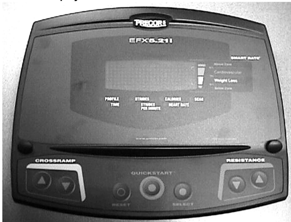
3. Watch the display as the LED test progresses. The test is programmed to display the following LED illumination sequence:
