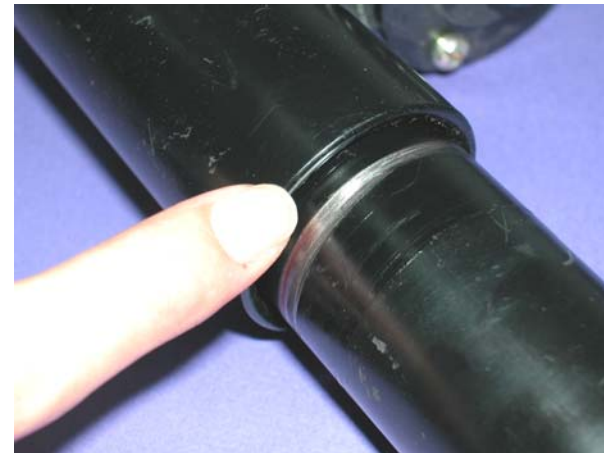
Step 2. Turn the incline motor pipe until the red line on the thin pipe is visible just above the end of the thick pipe.
