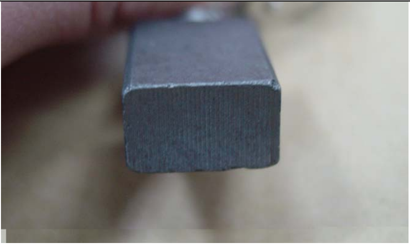
Illustration: Normal brush wear on a good brush
