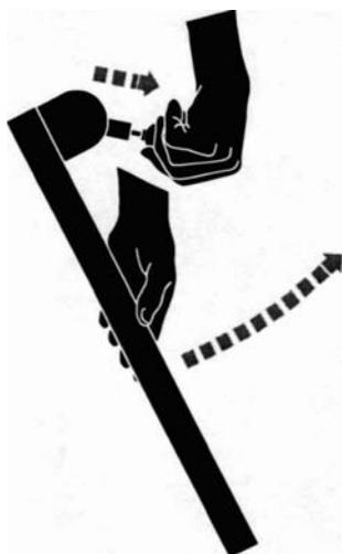
Pull the pin out to unlock the handle
